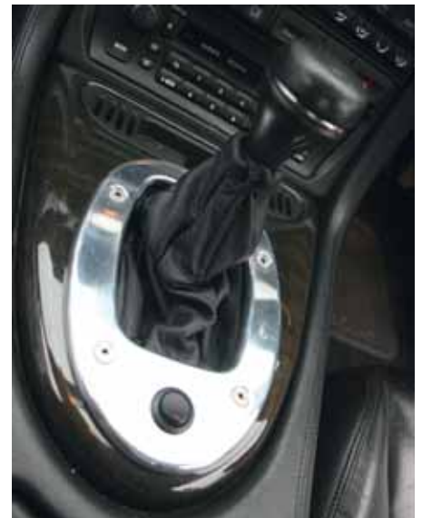
The non-standard gearlever gives the game away. The installation is tidy, and the button set into the surround needs to be flicked on to select reverse
