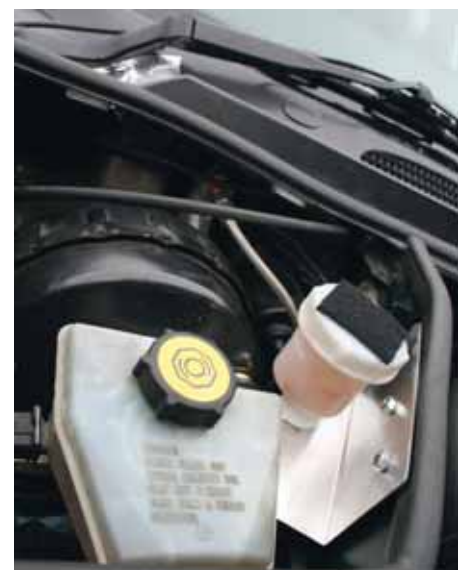
...remove the plastic cover on the off-side, however, and there's an XJ-S brake master cylinder and clutch fluid reservoir. A bespoke pedal box is on the way so final versions will not need the small hole cutting by the wiper blade – covered by the silver tape here
